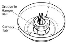
Figure 5b - Canopy Tabs and Grooves in Hanger Ball
